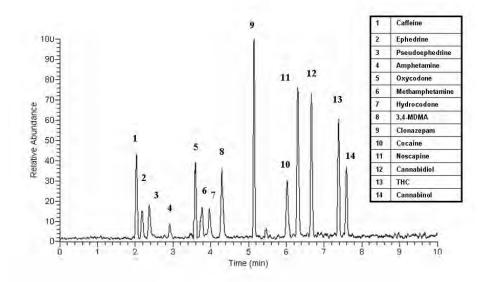
Figure1. UHPLC/MS chromatogram of 14 illicit drugs separated with ternary gradient.
